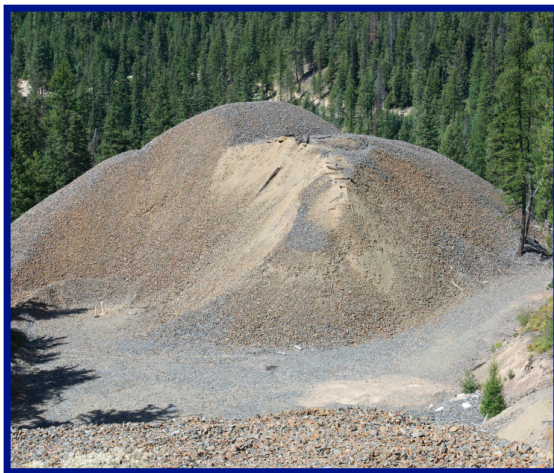
Mine Rock Waste Dump, 9 Mile Canyon
